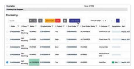
Once the part-program or configuration has been sent and the production process has been launched, the web app allows you to check the progress in real time, calculating the times, pieces and non conformities of each single machining operation.
