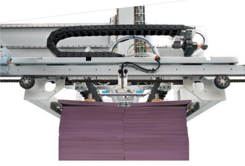
Guaranteed efficiency and reliability thanks to automatic set-ups and a piece detachment system for any type of panel stacks, both singe or double-row. It consists of slanted blades with integrated air jet, which, apart from ensuring panel detachment, guarantees the alignment of the panel stack at picking stage.
