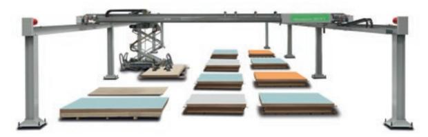
Winstore is an automated magazine for the optimised management of panels for large contract manufacturers, which guarantees production with reduced times and costs. Winstore can be integrated into nesting and sizing cells with a significant increase in productivity.
