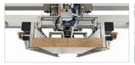
The gripper frame with pressor ensures grip over both single and double-row packs.
