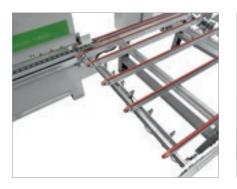
The sensors for the detection of the panel render the machine completely independent.
