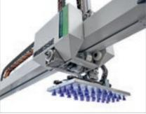
Withdrawal system for recirculation and unloading of panels with rotation. Automatic positioning via the dimension detection system.
