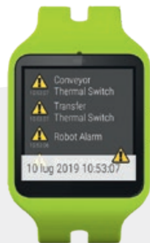
NOTIFICATIONS List of alarms or maintenance requests. Every time the machine signals that there is a problem, or when there is a maintenance request, the Viet Watch vibrates and a danger icon is displayed on the screen.
