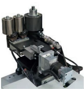
**Device for setting the unit automatically**, to suit the edging thickness (opt.).
