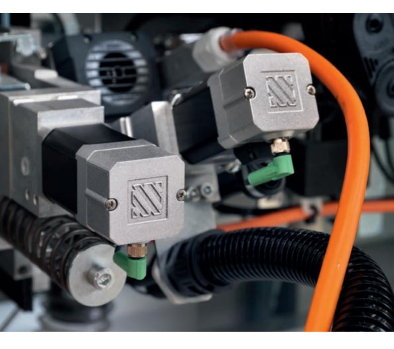
The automatic axis of the working units have a reading system that allows the machine to know -at any time -if the setting is correct. They are fitted with motors with a positioning tolerance of 0.01 mm, for optimum machining accuracy. Their compact size considerably extends their range of application. Changeover time reduced by 75%.
