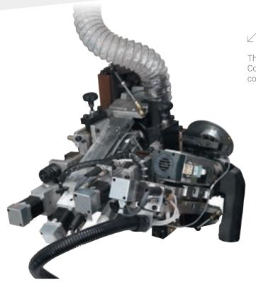
The Fine trimmer, for fine trimming of the top and bottom edges. Complete with 2 high-frequency motors and vertical/horizontal copiers with rotating disc.
