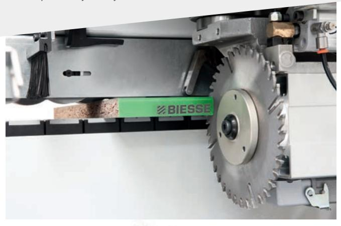
Reliability and cutting accuracy, due to the End Trimmer that removes excess edge at the front and rear of the panel. The Flex system, which is standard on the end trim automatically adjusts the excess edge whether the corner rounding unit is or is not being used.
