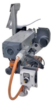
The **Grooving Unit** creates grooves and performs milling operations on the underside of the panel.
